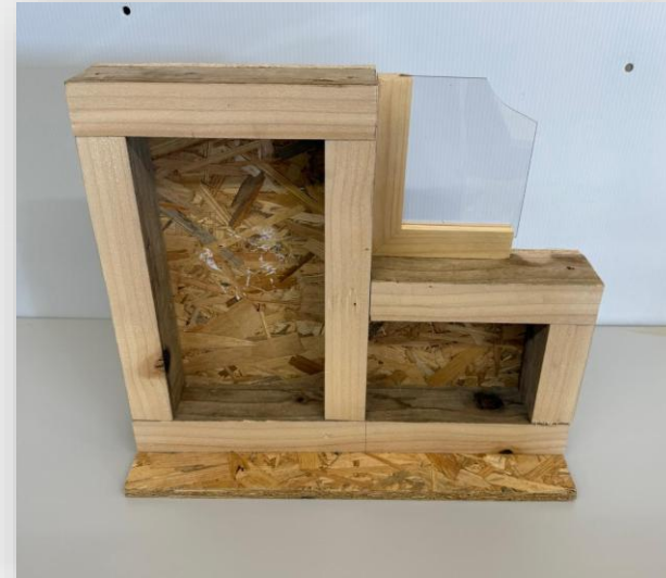
Model 2: Stud Partition with Widow Detail.
