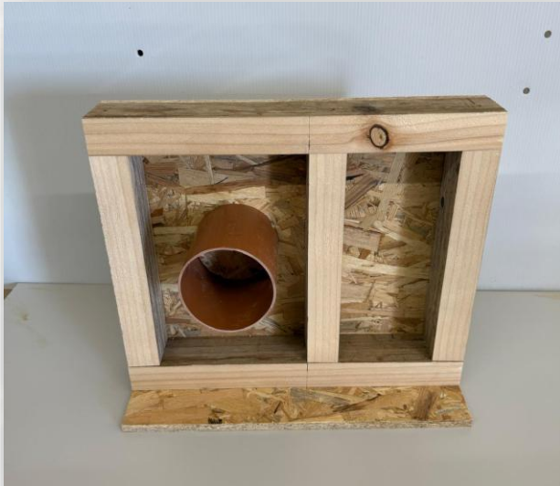
Model 1: Stud Partition with Waste Water Pipe & (LSF) Cable extruding
